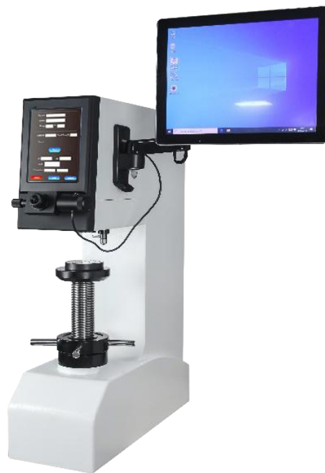
uBrin-3000M-V Auto-turret Vision Digital Brinell Hardness Tester
